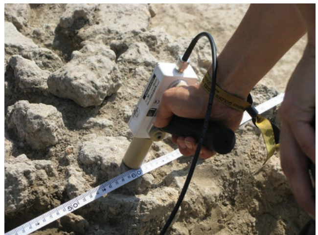
Fig. 3: Measuring of magnetic susceptibility
