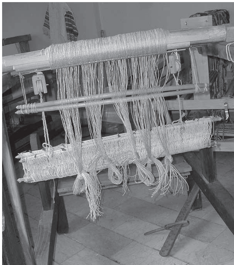
39 Wound warp before introduction into heddles
