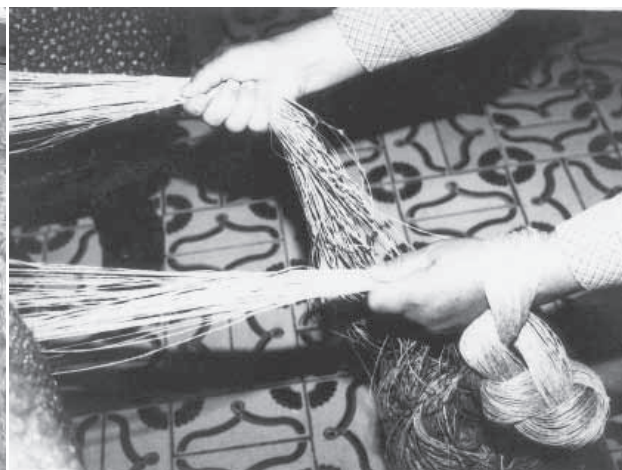
38 Counter tightening during winding on the back beam
