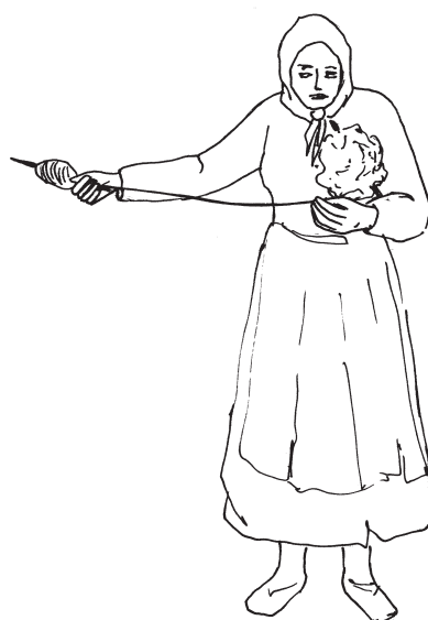
17, 17a Spinning with a elongated spindle in inclined position
