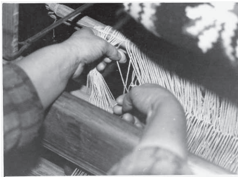
40, 41 Threading the first heddle
