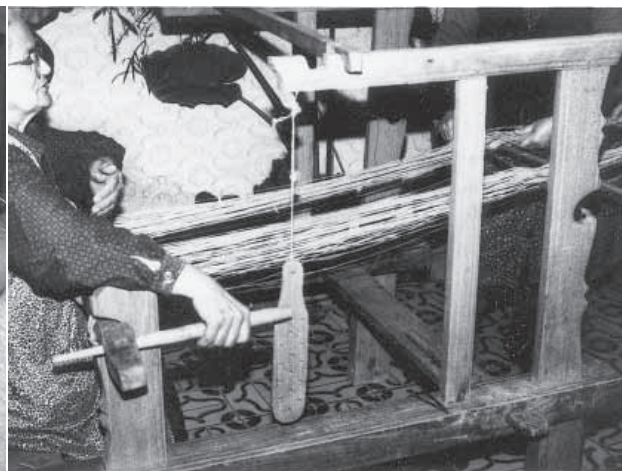
36 Winding of the warp on the back beam with a tightening mechanism
