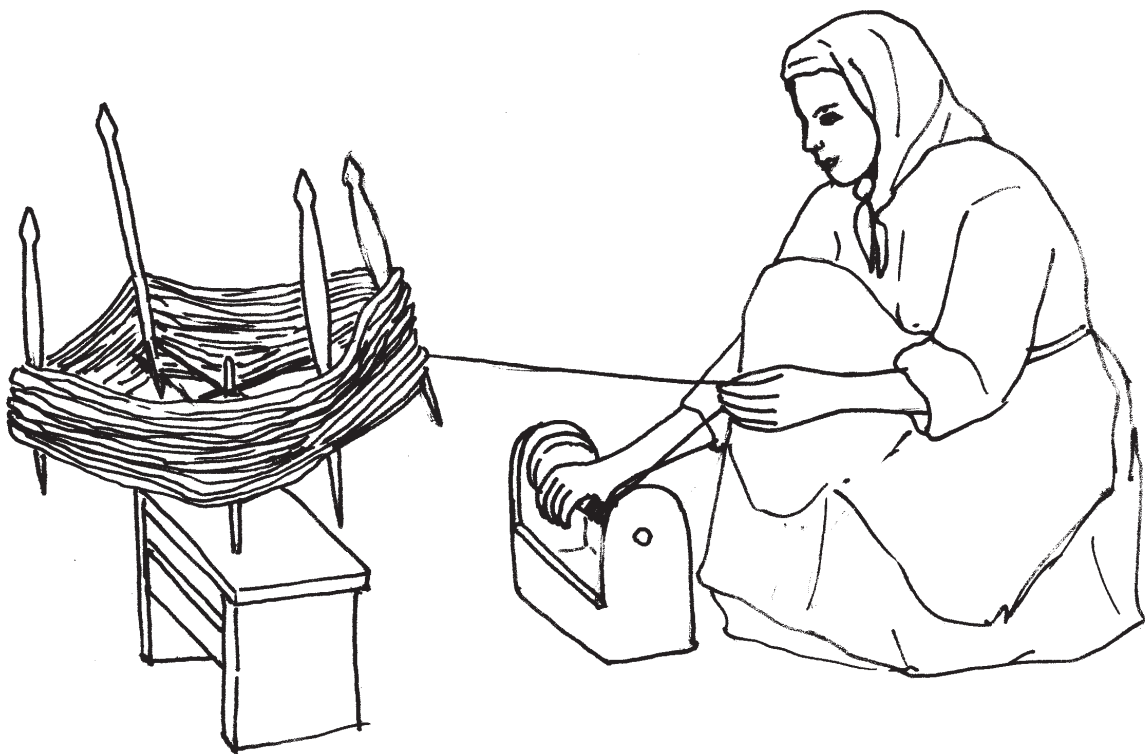
29 Rewinding of thread for the warp by a small respinner
