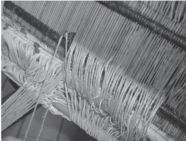
45 Introduction of the warp in the reeds
