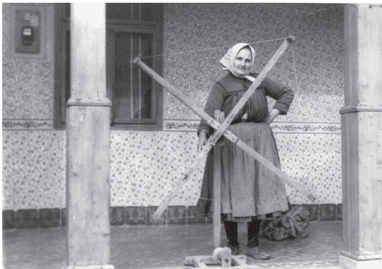
26 Winding of the hank on a cop with a cross wheel
